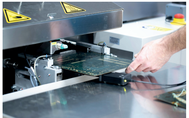
Reference board runs through the soldering system
